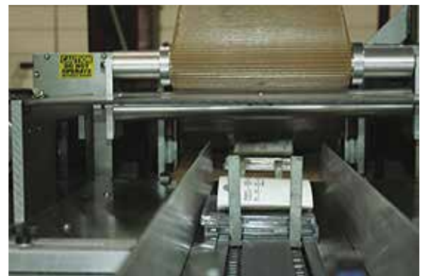
Stacked products comprising a small order, complete with return-policy and RFID-enabled labels, convey into one of two cohesive package-forming machines at Alliance Entertainment.
