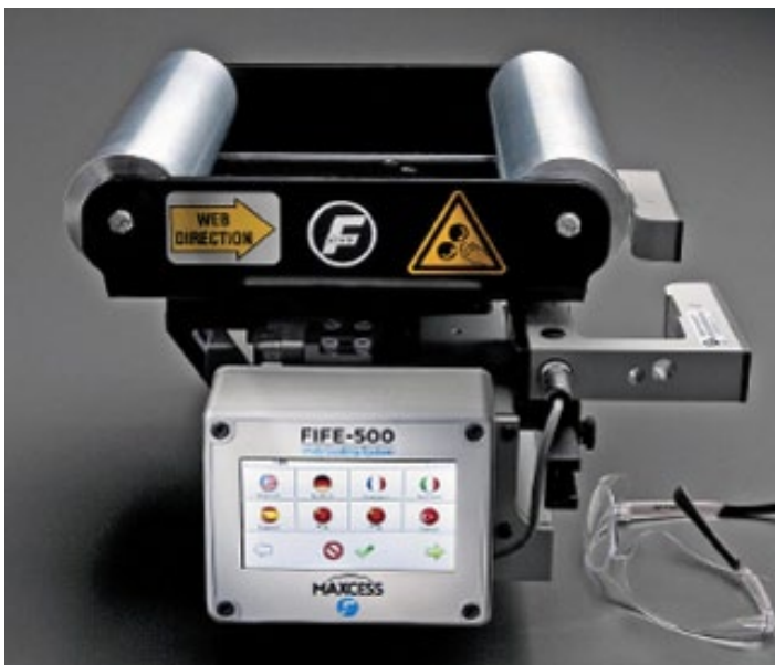
The film passes through ultrasonic sensors (extending from its right hand side in this photo) that detect the edges of the film, and a controller pivots the set of rollers to keep the web of labels perfectly in-line as they travel to the rewinder.
