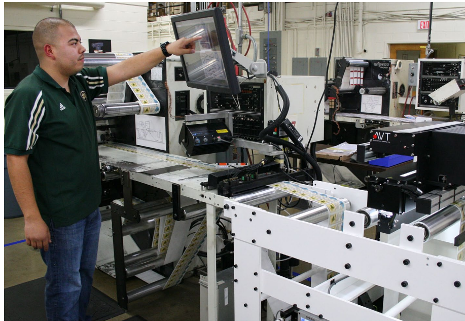
The incoming film is pulled through a series of rollers and travels to the Helios II unit where it passes between a light and the camera. The images from the camera are sent to the operator's screen. Any defects above the tolerance limits set by the operator cause the rewinder to stop.
